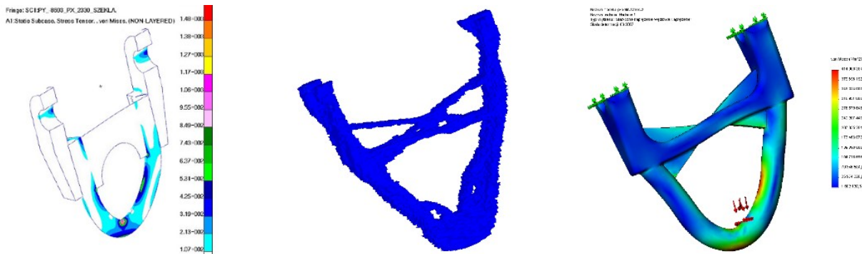
Figure 2. The biomimetic optimization of the shackle - from the left to the right: the initial configuration exceeded allowed stresses– the prototype , the optimization result, the final structural form of the shackle, after taking into account manufacturing constraints. Note, that the stresses are reduced below the assumed level.
